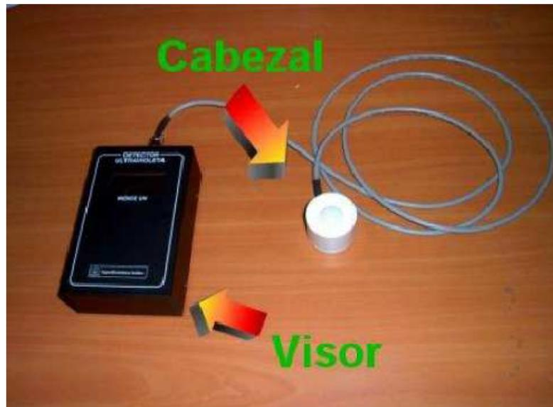
Figura 4.36: Medidor UV-A OPTO-360.
