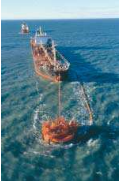
Figura 7, Terminal costa afuera con monoboya SPM (single point mooring buoy)
