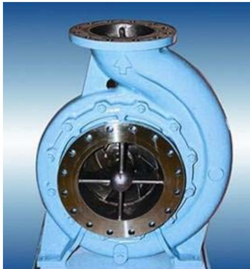
Figura 4.6: Bomba centrífuga C22BA
