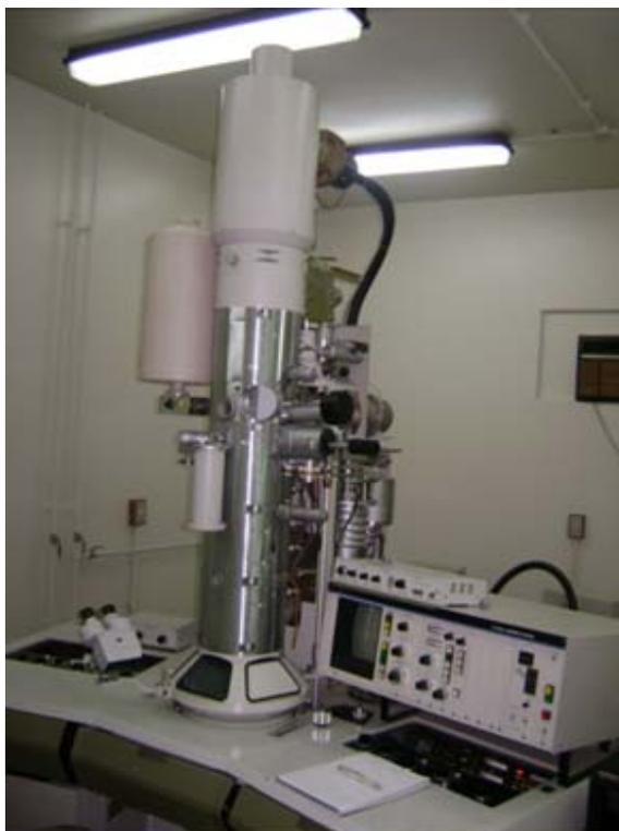
**Fig.6.9.** Columna Hitachi H-700h.
