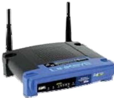
Figura 3.1: Router Linksys WRT54G v2.0
