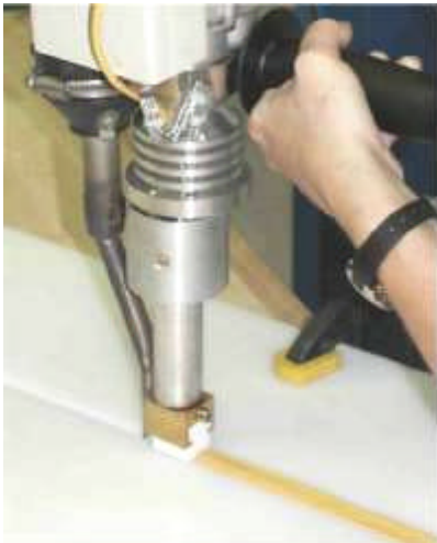
Butt weld performed with Mini extrusion welder on 'A" thick sheet
