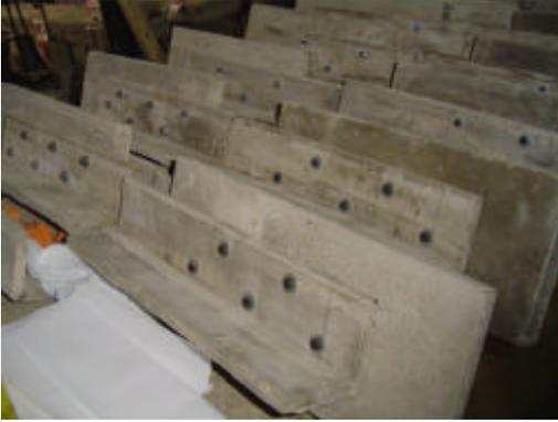
Fotografía 2.4 *Probetas con pernos*
